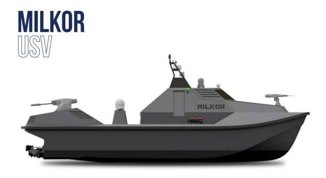
The Milkor USV is designed for various patrol missions and features dual remote control weapon stations, a 12.7mm weapon on the bow and a 30mm canon placed on the aft deck for potential threat engagement. Multiple VTOL systems are also included to provide operational oversight when needed.
