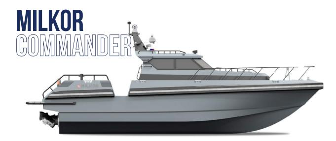
The Milkor Commander is a 16m Aluminium Monohull designed specifically for the needs of coast guards and law enforcement.
