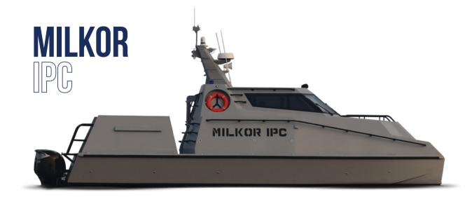
The Milkor IPC combines speed, stability and comfort to ensure consistent mission success. The unique design features a hydrofoil-assisted catamaran hull that increases speed, fuel efficiency and stability during operations. The vessel is designed for long-endurance missions featuring a full galley, shower, head and three sleeping berths creating a comfortable mission environment for its crew.
