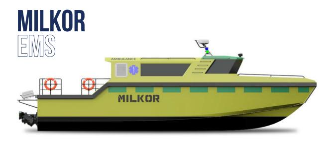
The Milkor EMS is a 16m aluminum monohull designed specifically for rapid emergency response teams that operate in shallow waters and narrow local water ways with limited access.
