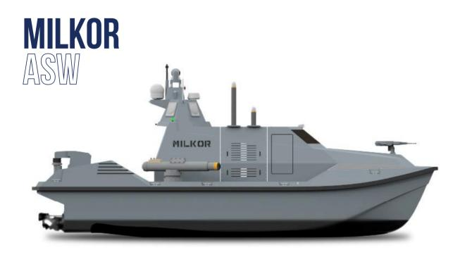
The Anti-Submarine warfare variant is suited for under water operations by detecting underwater threats through the use of a dipping sonar. To combat these threats, the ASW is fitted with side mounted torpedoes that enable the vessel to engage when necessary. As an additional protective measure, the vessel also features a surface-to-air missile system to eliminate potential airborne threats.
